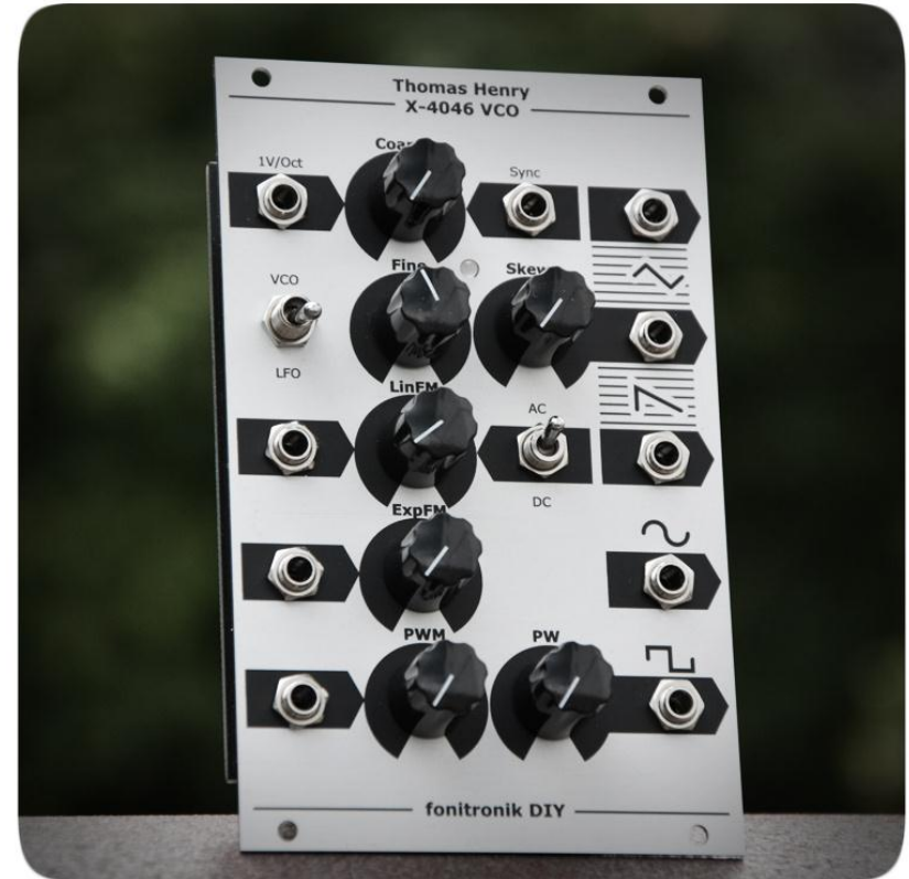
Prototype, built with the new main PCB and the additional eurorack adapter PCB.
